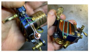
IT IS RECOMMENDED TO USE SILICON NIPPLES, OR VERY SOFT ONES FOR BETTER RESULTS. IT IS ALSO BETTER NOT TO USE ELASTIC BANDS WITH CARTRIDGE ADAPTER
